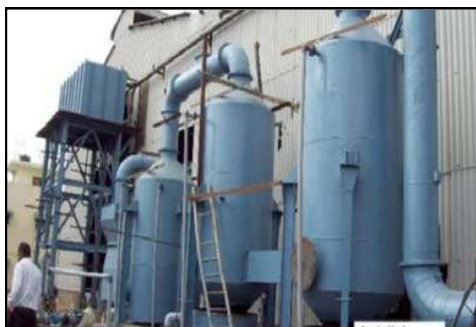
Four Stage Ventury & Scrubbing System
